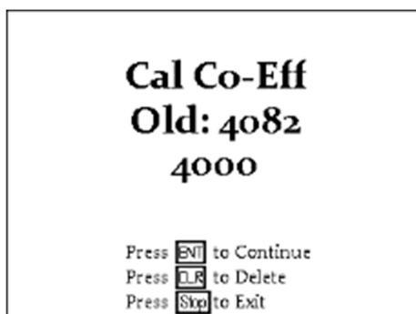
Record the Old calibration co-efficient on the calibration certificate, this will be needed to work out the new one.
