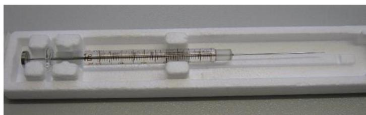
Injections of 10ul will be used during this calibration.
