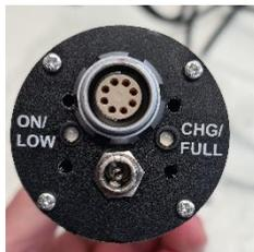
If the LED is lit red, then the unit should be put on charge. Use only the supplied charger to charge the unit (6V @2A max) – the unit will take 6-8hrs to fully charge.
