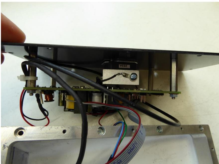
Remove the cover grille by unscrewing the 2 retaining screws at one end.
