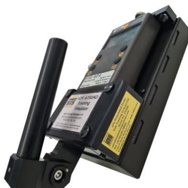
The STS ADK probe is a replica of a real Automess probe, but with additional STS electronics and batteries installed within the case. The unit is controlled by the 6150AD and turns on when the AD is turned on.
