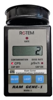
This simulator is a contamination **Only** variant – it does not work unless the cap is removed from the unit and only gives an output in CPS the Dose Rate -  $\mu$ S/h function does **not** operate although the red led will light up when the cap is placed on the unit.
