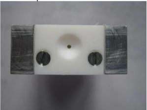
Reassemble the detector block by inserting the spring with the gauze end against the top of the detector and screwing the brass fitting back into place. Screw the brass fitting in slowly making sure that the spring doesn't deform and get
