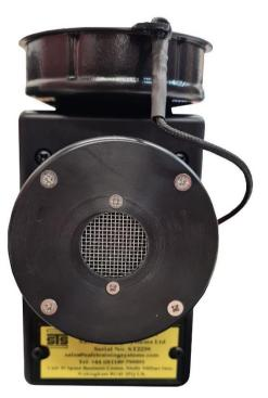
Looking at the perforated face plate of the probe remove the 4 screws through the cover and set aside.
