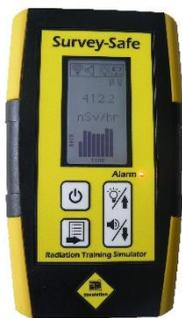
The STS Survey-Safe simulator is a simulated radiation survey meter designed to aid the tuition of workers in the nuclear industry in safe practices and in understanding the nature and mechanics of ionising radiation.
