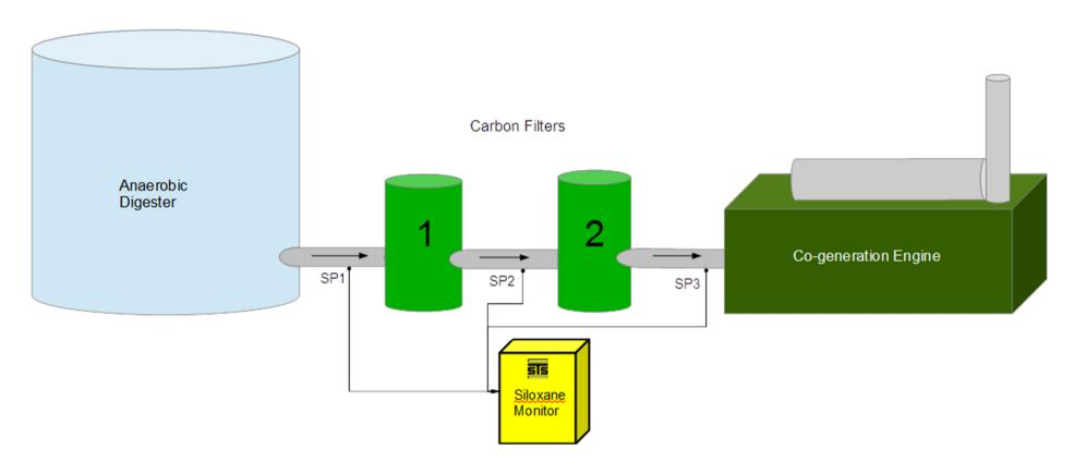
The STS Siloxane Monitor can sample from up to 3 points between the incoming gas stream and the engine. In typical application, these would be before the Activated Carbon filter (eg unfiltered gas), between a pair of filters where they operate a "primary and secondary" system and after the final filter (eg clean gas). The Monitor can therefore be used to trend filter use and predict filter failure and optimise filter change regimes.
