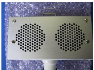
Looking at the perforated face plate of the probe remove the 4 screws through the cover and set aside.
