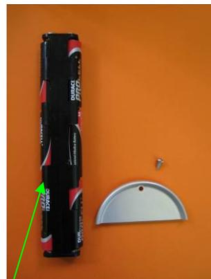
Replace batteries in holder with new AA cells
