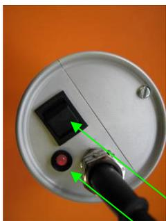
The SPA6 Probe is turned on by the switch on the top, the led will be lit green to show the instruments batteries are ok.
