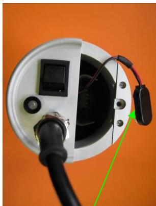
Undo battery clip and remove battery holder
