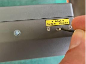
In Gamma mode the unit displays the reading form the source in USV with no probe connected or if the Gamma probe is connected it will additionally display EXT to show that the reading is from the probe and not the internal detector.
