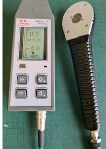
The unit is powered by a Lithium cell that will require recharging with the supplied charger by plugging in as below. The red led will light to show the unit is charging and will turn green when fully charged.
