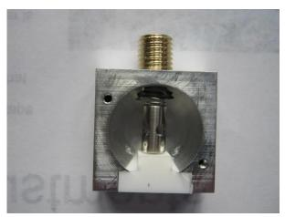
Unscrew the two screws through the white plastic block and carefully ease the detector
