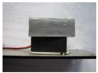
Align the detector plate and then the perforated face plate with the holes in the probe body and replace the 4 screws.
