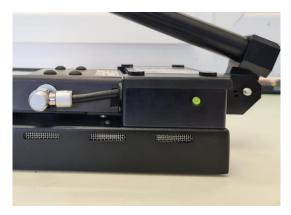
The ADK probe is powered by a pack of 6 AA cells housed in the black box at the rear of the probe. The probe is automatically turned on when the probe is connected to the meter and the meter is powered on.
