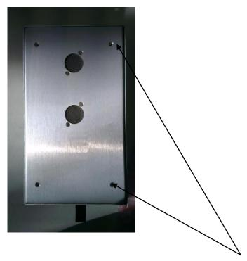
Looking at the face plate of the probe remove the 4 screws through the cover and set aside.
