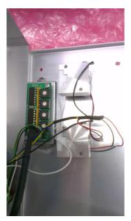
Once removed carefully undo the two screws through the detector plate. Before complete removal note the correct assembly of the components held by the screws. Remove the screws and carefully set aside the wire gauze and spacer, move the fan from the detector block to expose the brass tube mounted in the side of the detector.
