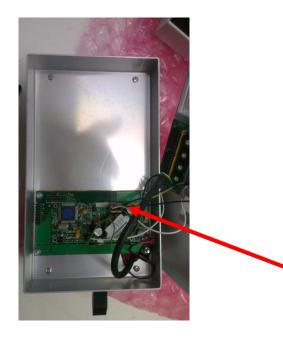
Carefully lift the detector plate from the probe body and disconnect the <u>5 way</u> connector mounted on the circuit board. Care must be taken not to remove this by pulling on the wires which may cause damage.
