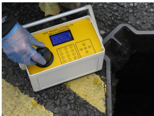
The SMF4 uses disposable 5ml plastic cells.
