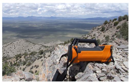
Devices communicate with the computer via USB or Bluetooth. The devices are powered by four AAsize NiMH recharge-
