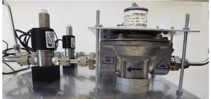
*The Siloxane Monitor can be used to monitor up to 3 incoming sample lines*
