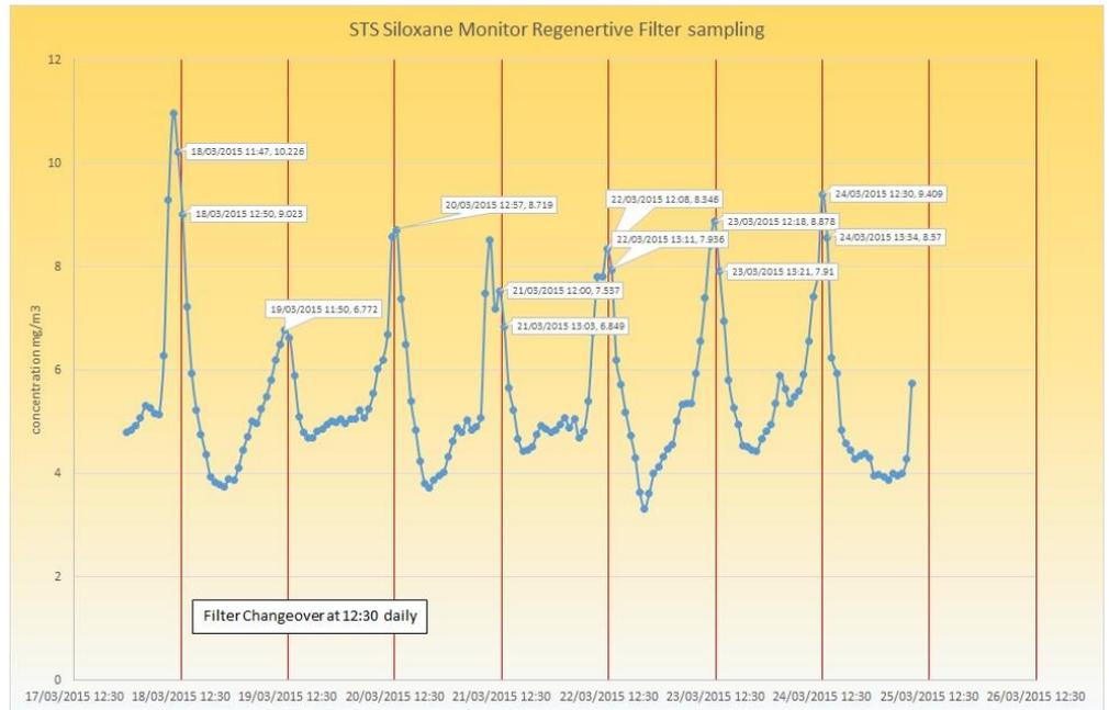
The Siloxane Monitor may be used for the optimisation of regenerative filter regimes ensuring that the maximum capacity of the filters is used before regeneration takes place. Cost efficiencies can therefore be made saving on the frequency of expensive regeneration, the data will also give advance warning of a deterioration of the filter media and therefore less efficient siloxane removal.
