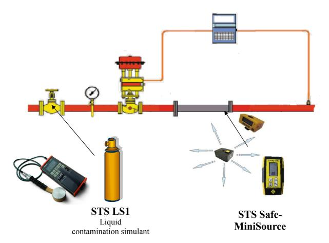
This training scenario is designed to use both the STS contamination and radiation simulators in the identification of a leaking valve generating a radiation field and a subsequent contamination of the pipe work and surrounding area.
