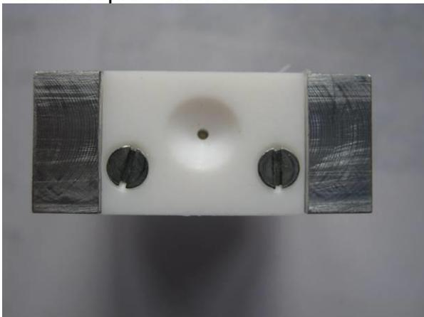
Reassemble the detector block by inserting the spring with the gauze end against the top of the detector and screwing the brass fitting back into place. Screw the brass fitting in slowly making sure that the spring doesn't deform and get trapped.
