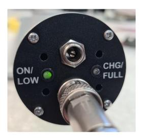
If the Led is lit red then the unit should be put on charge. Use only the supplied charger to charge the unit (6V @2A max) – the unit will take 6-8hrs to fully charge.
