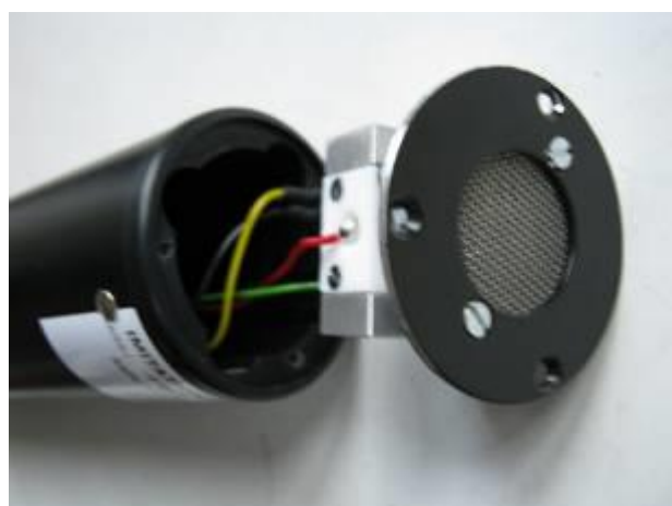
Slide out detector assembly
