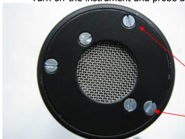
Undo 3 outer retaining screws
