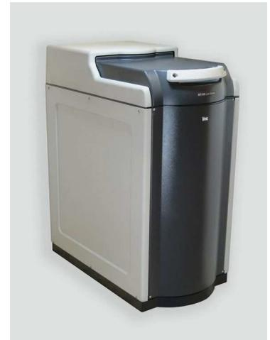
**In steel samples the final accuracy of the measured contamination is as low as 0,02 Bq/g using a measurement time of only 5 minutes.**
