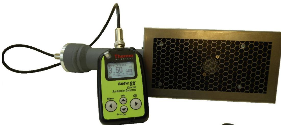
STS are pleased to announce the launch of the first ever simulated probe to work with an unmodified Thermo RadEye SX. The new smart probes connect via a standard BNC cable to a users existing RadEye which retains its full functionality. The probe automatically turns on when the RadEye is powered on and utilises STS's highly successful gas simulation system.
