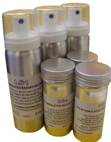
The liquid source material (LS1) is transferable and so is ideal for demonstrating the hazards of cross contamination from surfaces to clothing and equipment. The contaminated surface may be cleaned using standard methods and then re-monitored to demonstrate effective decontamination techniques.
